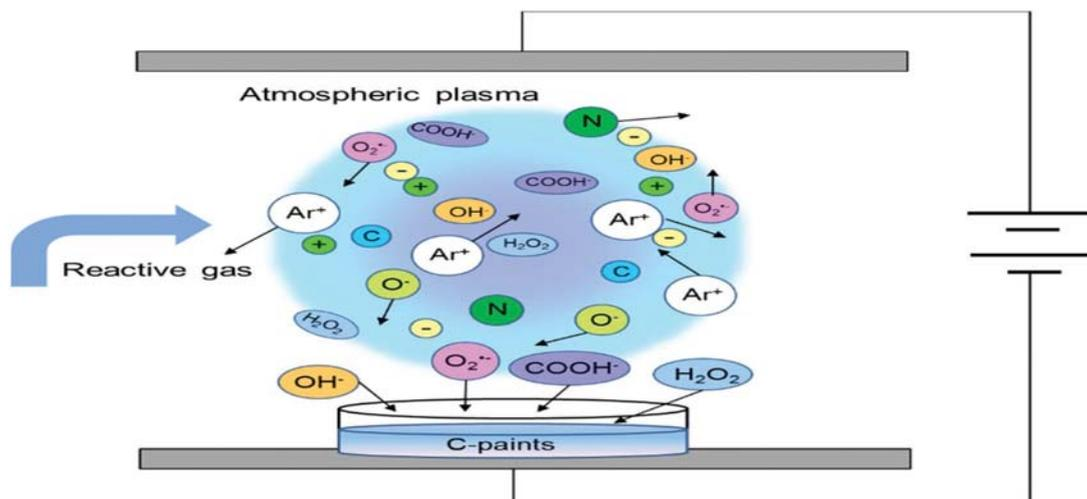
**Scheme 1** Schematic of plasma reaction with C-paints. Atmospheric plasma treatment resulted in the formation of functional groups on the surface of C-paints to fabricate AC-paints. On addition of reactive gases involving oxygen or nitrogen, organic molecules or reactive oxygen species were formed on the surface of C-paints.
