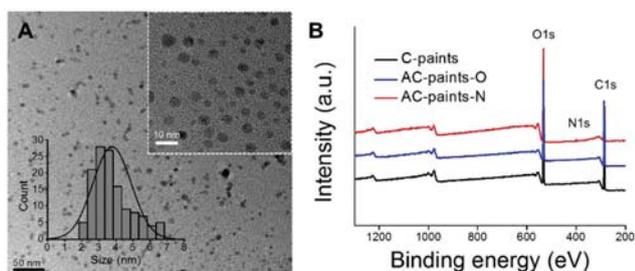
**Fig. 1** Characterization of C-paints and AC-paints. (A) TEM images of AC-paints-O after oxygen plasma treatment of C-paints. Inset shows size distribution of AC-paints-O, (B) XPS spectra of C-paints and AC-paints ( $O_2$  and  $N_2$ ).
